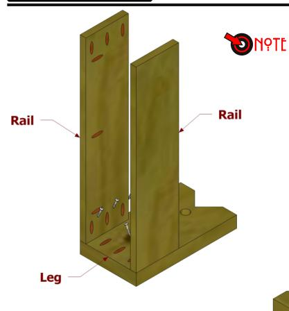
Position the parts as shown at left and below and attach using glue and 1 1/4" pocket hole screws.
