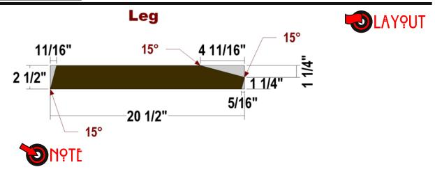
Use the layout as a guide to create the Legs. For the taper at the end, you can either use a table saw and a tapering jig, or a jigsaw.
