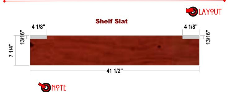
Use the layout as a guide to create the Shelf Slats. Use a jigsaw to cut the notches.
