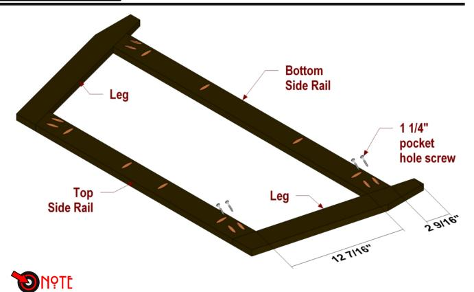
Apply glue to the ends of the Top Side Rail and Bottom side Rail, and position the parts as shown. Attach using 1 1/4" pocket hole screws. Create two assemblies.
