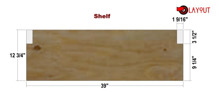
STOTE Use the layout to create the Shelves. Use a jigsaw to cut out the notches.
