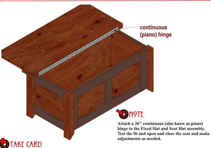
Attach one or two lid supports to prevent the Seat Slat assembly from slamming shut, particularly if you have small children around.
