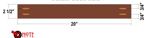
Use the layouts for creating the Top Back Rail, Bottom Back Rail, Outer Back Stiles (two), and Center Back Stile. Set your Kreg Jig and drill bit for 3/4" stock.
