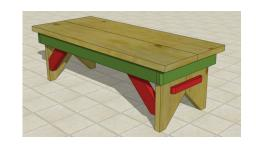
2x12, 2x10, 2x4, 2x2 3-inch deck screws 2 1/2-inch deck screws miter saw/circular saw drill/driver
