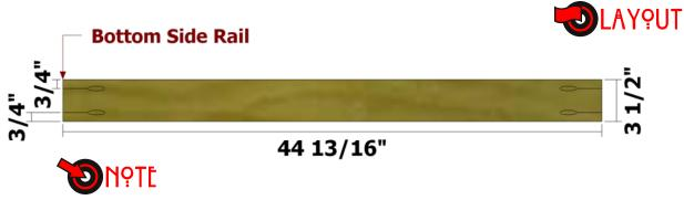
Use the layouts above for creating the Bottom Side Rails. Set your Kreg Jig and drill bit for 1 1/2" stock.
