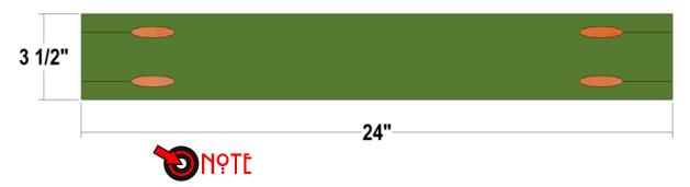
Use the layout for creating the Stretchers and Side Rails. Set your Kreg Jig and drill bit for 1 1/2" stock.
