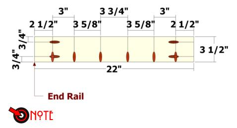
Use the layouts for creating the Legs and End Rails. Set your Kreg Jig and drill bit for 1 1/2" stock for the pocket holes on the End Rails.
