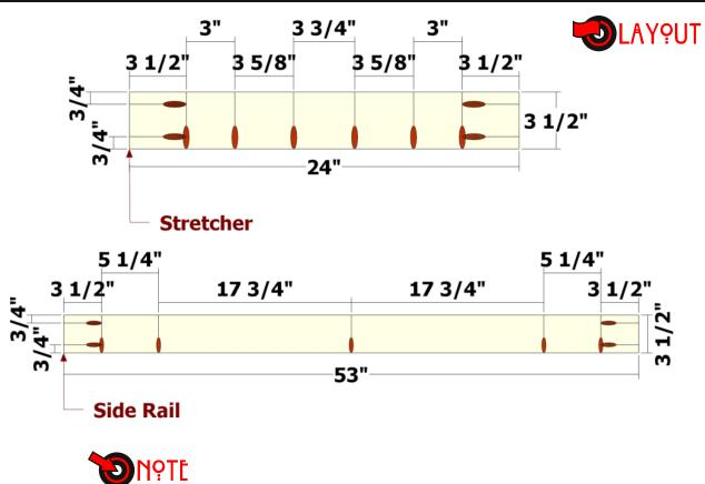
Use the layouts for creating the Stretcher and Side Rails. Set your Kreg Jig and drill bit for 1 1/2" stock for the pocket holes on both parts.
