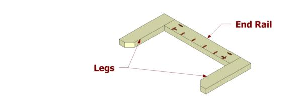
Position the parts as shown and attach using glue and 2 1/2" pocket hole screws. Create two assemblies.
