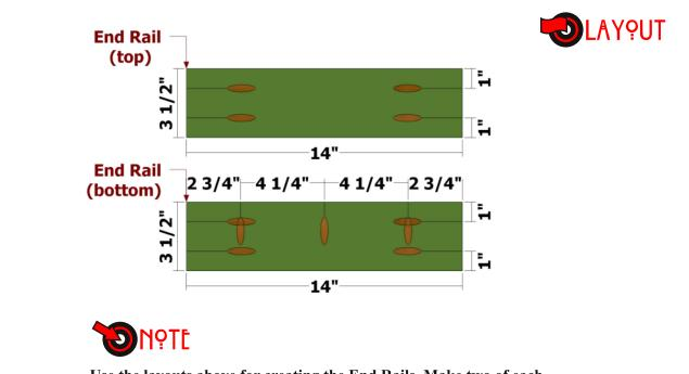
Use the layouts above for creating the End Rails. Make two of each layout. Set your Kreg Jig and drill bit for 1 1/2" stock for the pocket holes on the ends (horizontal), and for 3/4" stock for the vertical holes.
