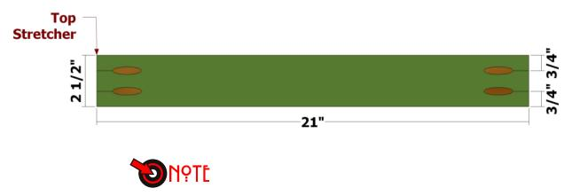
Use the layout above for creating the Top Stretcher. Set your Kreg Jig and drill bit for 3/4" stock for the pocket holes.
