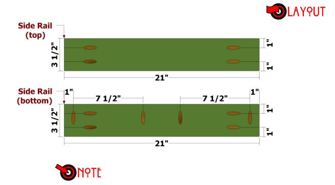
Use the layouts above for creating the Side Rails. Make two of each layout. Set your Kreg Jig and drill bit for 1 1/2" stock for the pocket holes on the ends (horizontal), and for 3/4" stock for the vertical holes.
