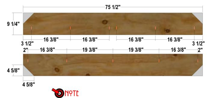
Use the layout for creating the Slats. Set your Kreg Jig and drill bit for 1 1/2" stock. Each angle on the parts is cut at 45 degrees.
