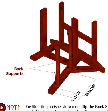
Position the parts as shown (or flip the Back Supports over so the pocket holes are facing down) on this page and attach using glue and 2 1/2" pocket hole screws.
