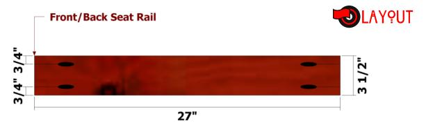
**Source** Use the layout above for creating the Front and Back Seat Rails. Set your pocket hole jig and drill bit for 1 1/2" stock.
