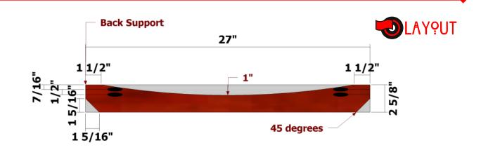
Use the layout above for creating the Back Supports. Set your pocket hole jig and drill bit for 1 1/2" stock.
